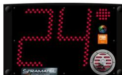
Horn loudness (115dBa at 1m): ⚠ the high sound pressure can deteriorate hearing. Therefore, the spectators should be kept at a reasonable distance from the display units. The horn is not equipped with the possibility to adjust the loudness of its sound.
