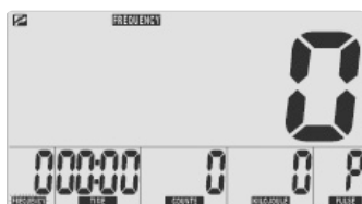
Figure 4 Ready for training: frequency flashing
