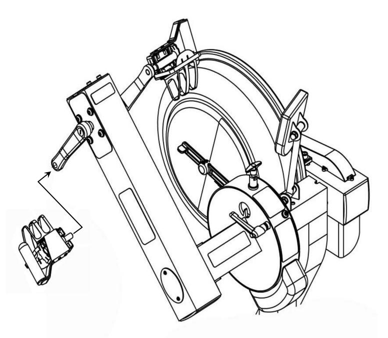
**Step 5:** Secure right pedal onto Crank arm. The pedal threads have a blue coating which will feel very tight when threaded onto the crank arm. This is a type of thread locker, and once in contact with the crank arm threads will activate in approximately 15minutes.
