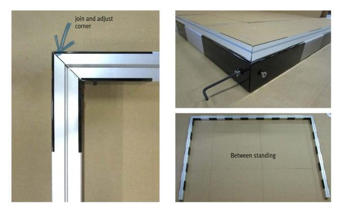
**Advice:** Due to production tolerances of the aluminium cast corner joints problems during adjustment of corners may possibly occur. Then shorten the stamps in the uprights with a flat file.
