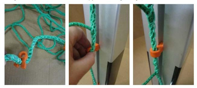
c) Dismantling of the net is also done by rotation of the net holders through 90 degrees. Use again a thin screw driver if necessary.
