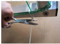
d) Cut the attached cord in half so that there are 2 short cords. Fix the end of one cord in one upper ring nut and knot it well. Pull the cord through the net meshes and fix it in the 2nd upper ring nut and knot it well.
