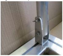
i) Stick ring nuts M 6 x 50 through boreholes of the net hoop (position see picture below) and fix them with washer DIN 9021, 7.4 x 22 and self-locking cap nut DIN 986, M 6. **Take care that rings point to the inside.**
