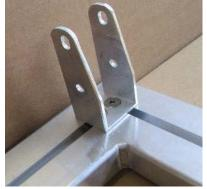
c) To fix the lower hinge stick from the bottom (upright's end) 1 nut 20 mm, M 8 each in the guide rail of the upright. Mount lower hinge with 1 fastening borehole.
