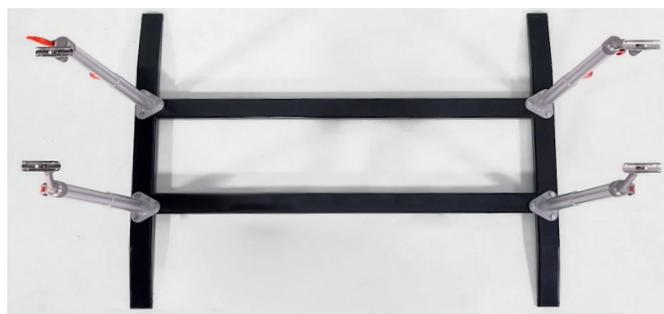
**3.** Place the rails (D) with the pre-drilled holes on the therefore dedicated dishes. Mount each rail with 8 countersunk socket head screws M6 (G). The M6 screw must be mounted with the included allen key size 4. Pict. 4 +5
