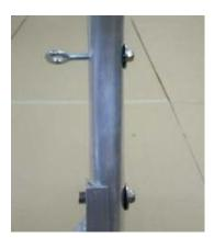
e) Stick from the inside ring nuts M6 x 50 for tensioning net rope through the open boreholes of both net hoops and fix with washers DIN 9021, 7.4 x 22mm and nuts DIN 985, M6.
