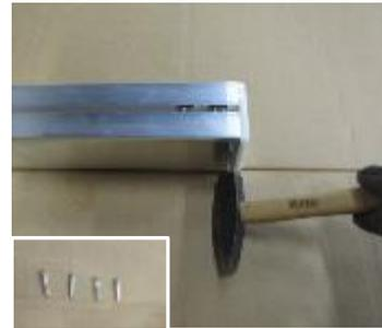
Lay ground tube on the ground with groove facing upwards. Push 2 nuts 20mm, thread M8 into the groove of each ground tube and place ground tube between the ground bars. Then place connecting plates (flat plates with 4 holes) and push already mounted nuts below the connecting plates. Stick at each side 4 spring washers A8, DIN 127 on 4 hexagon socket screws M8 x 20, DIN 933 and screw them slightly into the nuts at ground tube and ground bar.
