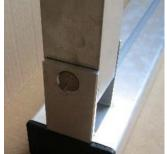
f) Fixing of the hoop at the upper hinge: Stick from the top hexagon screw DIN 933, M 8 x 60 through the first borehole of hinge and hoop. Then add washer DIN 125, Ø 8.4 mm at the hinge lower side, screw and tighten self-locking nut DIN 985, M 8. Fixing of the hoop at the lower hinge: Stick from below slotted countersunk head screw DIN 963, M 8 x 60 through hinge and hoop. Then add washer DIN 125, Ø 8.4 mm at the hinge upper side, screw and tighten self-locking nut DIN 985, M 8.
