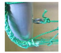
d) Cut the attached cord in half so that there are 2 short cords. Fix the end of one cord in one upper ring nut and knot it well. Pull the cord through the net meshes and fix it in the 2nd upper ring nut and knot it well. Repeat the steps with the 2nd cord in bottom ring nuts.
