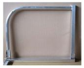
Fix net hoops in the hinges. Take care that the end of the net hoop with 2 boreholes e) (round tube) is fixed in the upper hinge and the end with 1 borehole (square tube) is fixed in the lower hinge. Boreholes of hoops have to be congruent with boreholes of the hinges.
