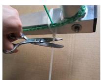
c) Fix net at the bottom of net hoops with 3 cable clips. Cut projecting parts.
