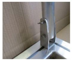
h) Press net hoop to the outside. Stick from the top hexagonal screw DIN 933, M 8 x 60 through the 2nd borehole of the upper hinge and the hoop. Then add washer DIN 125, Ø 8.4 mm at the hinge lower side and screw wing nut DIN 315, M 8.
