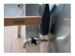
Use a hammer or mallet to fix the grooved pin 3 x 20mm in the hole of the composed stick so that it projects equally at both sides.
