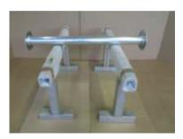
Place reel tube on a suitable construction (supports, table or similar, height approx. 600 mm).
