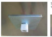
Stick 1 washer  $\emptyset$  outside 44 mm, DIN 126 and then 1 polyamide liner 40 x 40 mm on the plugs.
