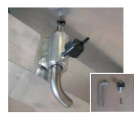
Push from the outside composing stick  $\emptyset$  9mm through the sleeve hole and fix it with a wing bolt M8 x 16.
