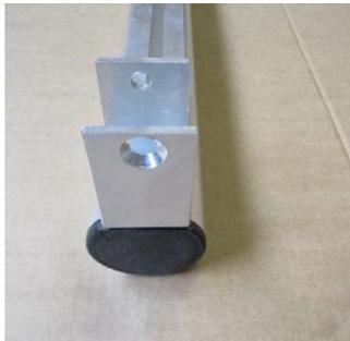
d) Beat cap 80 x 40 into the upright (use a mallet if necessary), adjust lower hinge and tighten fixing screw. Take care that the hinge at the bottom is flush with the upright's cap.
