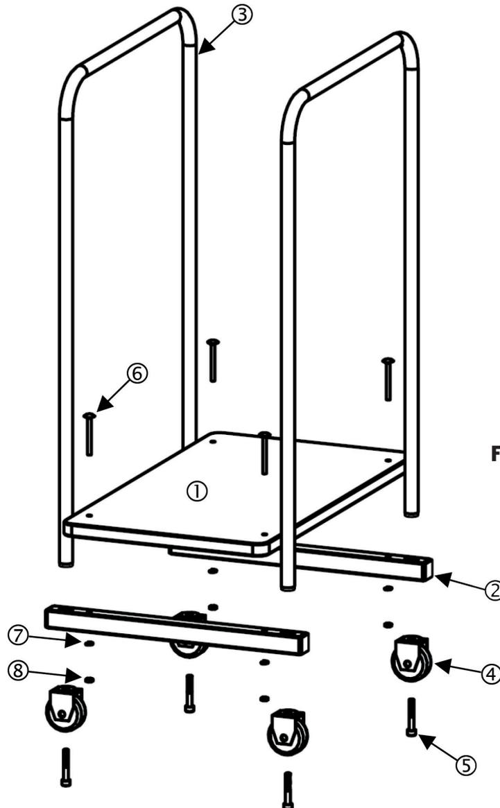
**Figure 1: Assembly plan**
