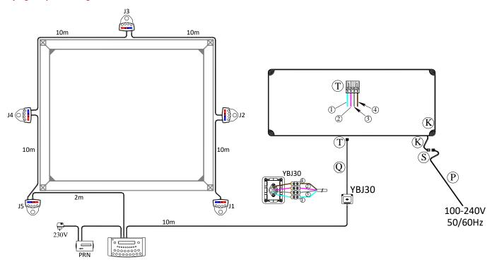
Control cable (Q): (1) = GND = blue wire / (2) = Rx+ = white wire / (3) = Rx- = grey wire / (4) = +24V = transparent wire
