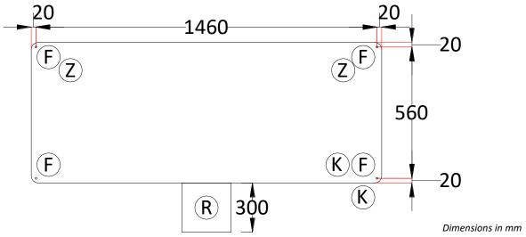
(Z): Holes for mounting or disassembling the front face in some maintenance cases.
