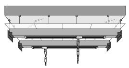
suspended ceilings, a laminated beam must be mounted underneath the concrete ceiling between two beam wall holders. Ensure, that the maximum distance between the walls is 6 m. The walls must be solid.
